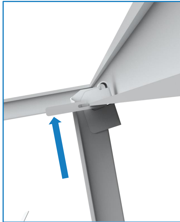
Slide the Frame Enhancer along the Tilt Arm. Stop when the Frame Enhancer is in contact with the bottom of the module flange.
