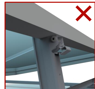
LOCK CLAW NOT INSTALLED
