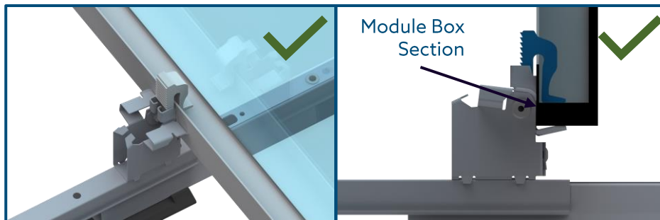
Example of a good installation of the Cam Claw. Cam Claw is straight and is in contact with the inside of the Module frame
