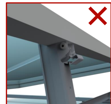
LOCK CLAW NOT INSTALLED
