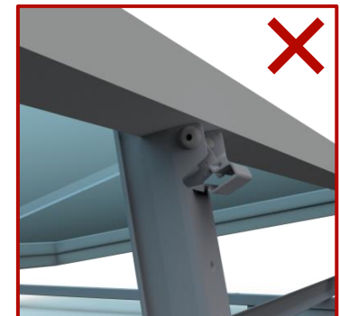
LOCK CLAW NOT INSTALLED
